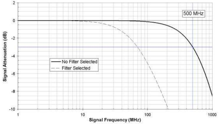
Note: Typical Frequency Response curves above taken on the  $\pm 1$  V input range with 50  $\Omega$  termination and DC coupling. In AC coupling mode, the lower -3 dB cutoff is at 20 kHz.
