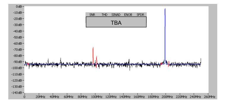
Frequency spectrum above taken on an EON CompuScope on its ±500 mV input range with DC coupling.
