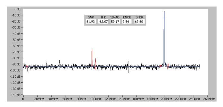
Frequency spectrum above taken on a CS12501 on its ±500 mV input range with DC coupling.
