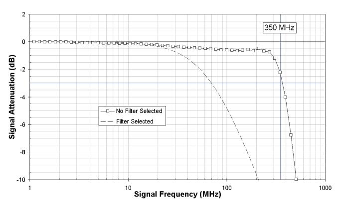
Note: Typical Frequency Response curves above taken on the  $\pm 500$  mV input range with 50  $\Omega$  termination and DC coupling. In AC coupling mode, the lower -3 dB cutoff is at 20 kHz.
