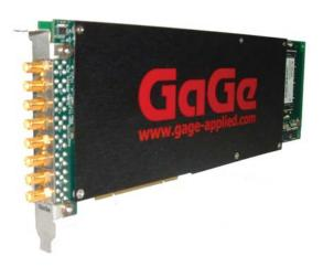
The Razor family of 12-bit digitizers represents a new generation of high-speed, high-resolution data acquisition cards from GaGe. Razor digitizers offer many powerful advanced features including:
