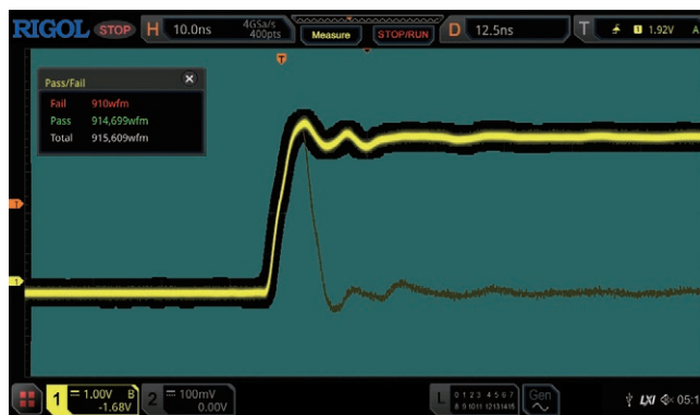
The Pass/Fail test function can quickly make a statistics on the occurrence probability of the signal exceptions.
