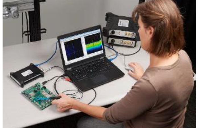
FIGURE 11. The DPX real time spectrum analysis with a near field probe helps you discover and locate the transient emission sources.
