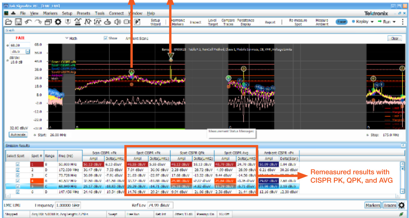
FIGURE 8. Re-measure the selected over limit spurs with CISPR quasi-peak and average detectors.
