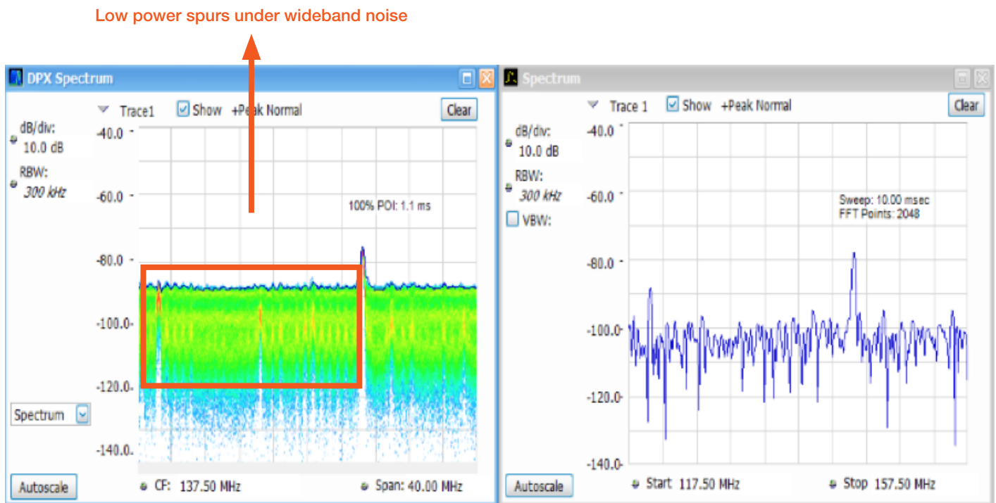
FIGURE 12. The DPX real time spectrum analysis vs regular swept spectrum analysis. DPX can detect transient signals, and helps users to gain insights of co-channel interference.
