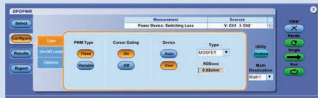
Figure 7. The DPOPOWER input page allows the user to enter data sheet values for R_{DS_{ON}} & V_{CE_{sat}} .
