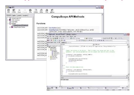
Gage's CompuScope C/C# SDK allows complete control of Gage CompuScope hardware from a C/C# application running under Windows. The SDK provides several C and C# sample programs illustrating the use of CompuScope hardware in different operating modes. These sample programming examples serve as a starting point for an optimized C or C# application using Gage CompuScope hardware.
