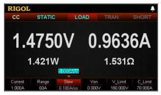
Current rising speed is defined as the speed of transition from one setting to another. You can set the actual transition time from one setting to another by changing the current rising speed. Adjustable current rising speed: 0.001 A/µs to 5 A/µs.
