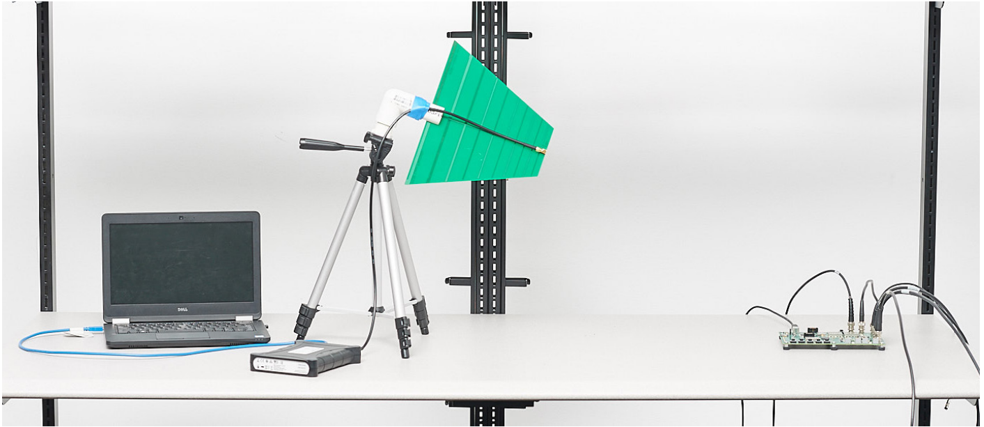
FIGURE 11. A typical troubleshooting test setup for radiated emissions. The distance between antenna and equipment under test is approximately 1m.
