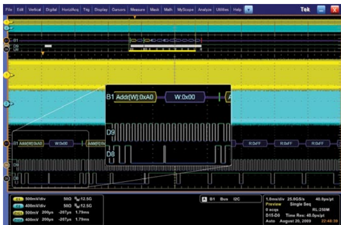
Figure 11. MSO70000 decodes address 0xA0 after crosstalk issue is resolved.
