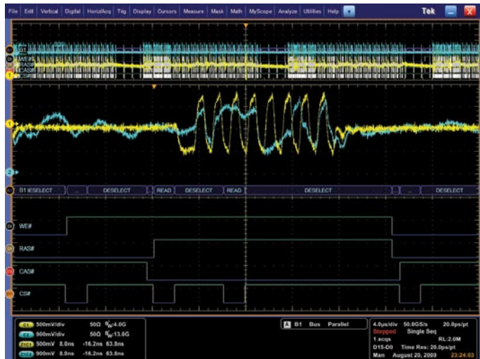
Figure 11. DDR3 Command Bus decoding on MSO70000.
