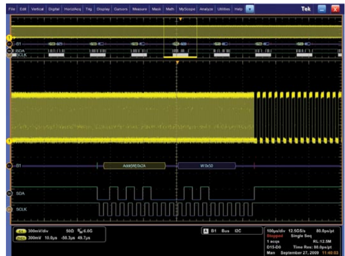
Figure 2. MSO70000 can provide time correlated views of analog and digital signals.
