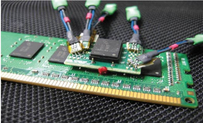
Figure 5. Component Interposer with solder tips; eye diagram of probed signal.
