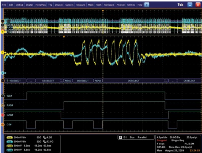
Figure 4. Bus qualified trigger of memory read cycle.
