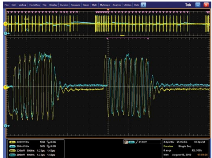
Figure 8. Using Advanced Search & Mark to identify all write bursts.
