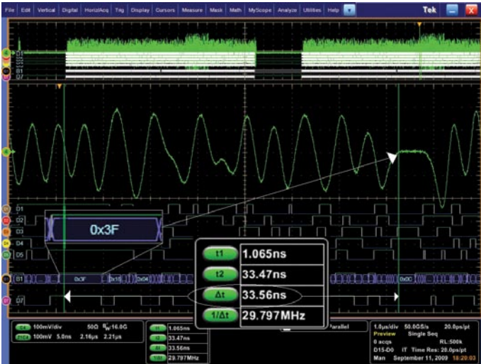
Figure 17. The integrated view of the logic states at the DAC and Analog output.
